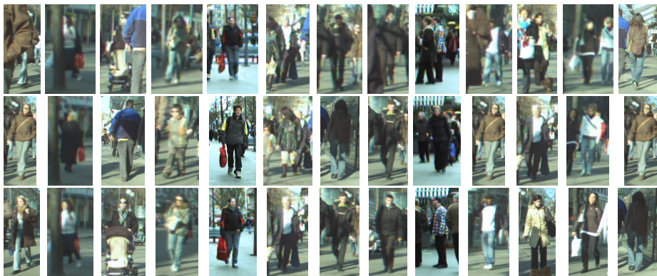
Fig. 4: Identity inference results (SvsAll). First row: test image, second row: incorrect NN result, third row: correct result given by GCIDInf.
