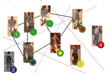
Figure 3: An example from 3DPeS: the outer circles on nodes indicate the correct class label, and the center of each circle the label given by the SVMs. Filled numbered circles are gallery images and dashed lines indicate the SVM margins. The SVM errors are all corrected by the CRF thanks to the local topology (black lines).
